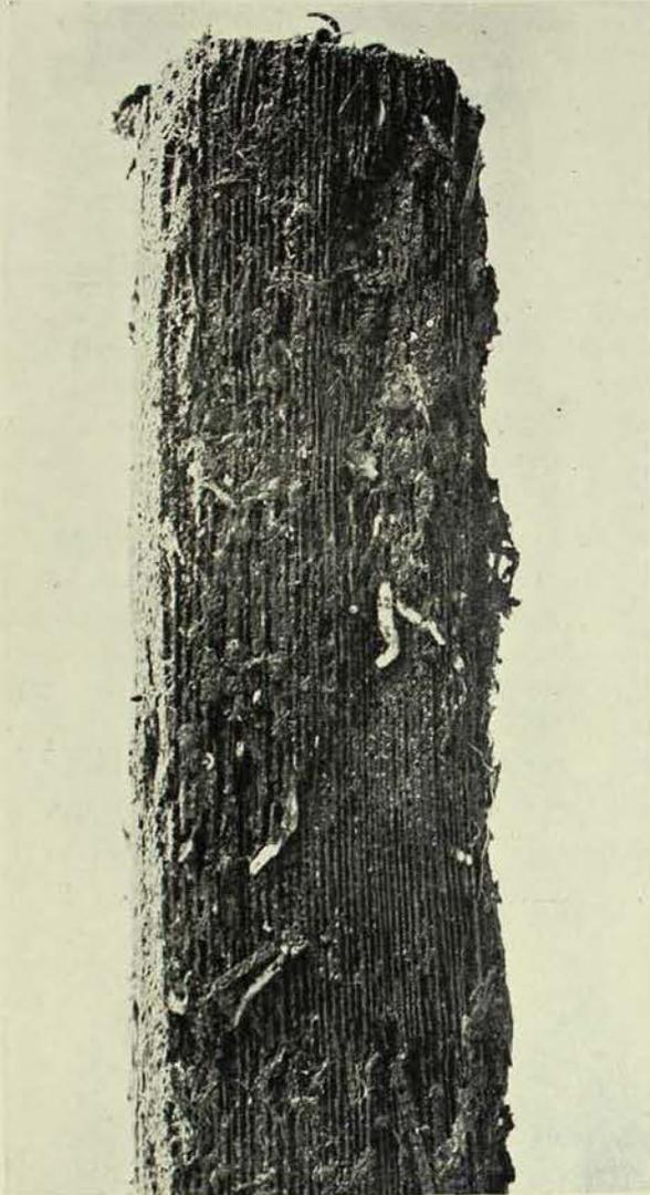
Same piece of wood showing external attack by crustacean pests, which in some parts has exposed the shell-lined tubes of the cobra.
