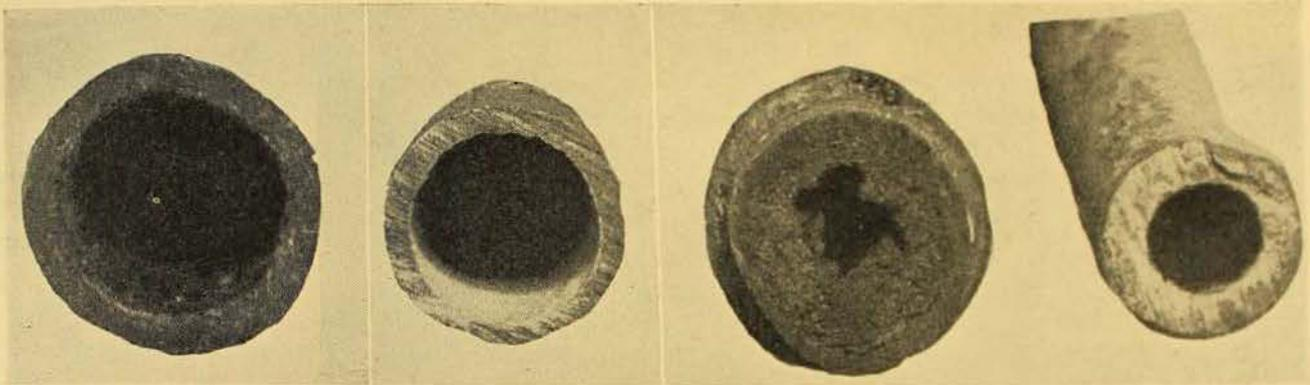
**End view of four water pipes. On the left is a new type of iron piping lined with bituminous compound to prevent the workings of iron bacteria. Alongside it is an unused iron pipe for comparison with the next one, which is regular iron pipe badly affected by iron bacteria. On the extreme right is an old style lead pipe; it is unaffected by iron bacteria even after seventy years of service.**
