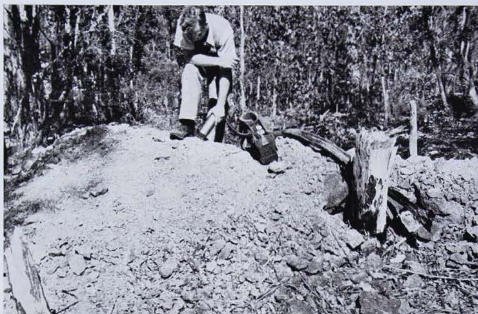
J. C. Lloyd, of the Geological Survey, uses a scintillometer to test the mullock heap alongside a disused mine shaft near Glen Innes.
