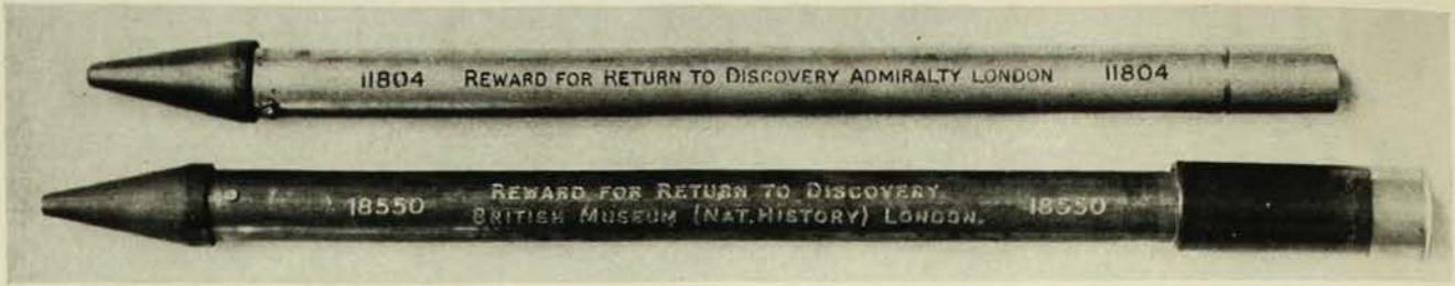
Below: A whale mark with its cartridge attached. This whole unit is inserted in the breech of a 12-gauge shotgun. Above: A mark after it has been fired. The whole mark enters the dorsal muscles of the whale and is recovered when the mammal has been killed and is being processed on a factory ship or at a shore station. [In the early days of whale marking marks were returned via the Admiralty instead of the British Museum (Natural History), as at present.]
