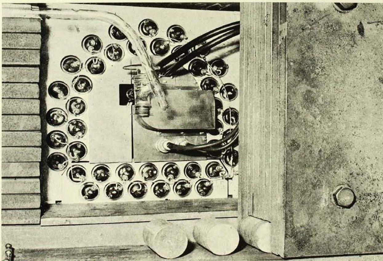
The iron door rolled back reveals the ends of a double ring of Geiger tubes. A glass tube and stopper admit gas to the counter tube.
