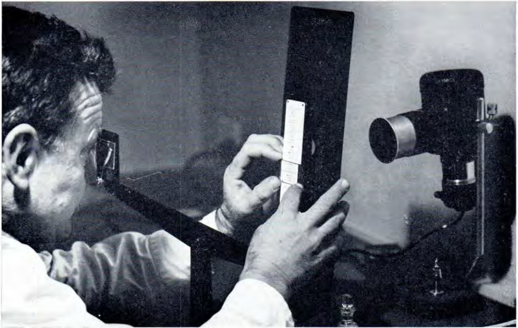
Research in the laboratory includes the study of specimens with instruments for measuring and recording a variety of characteristics. Here a mineralogist uses a Leitz-Jelley refractometer, which enables the refractive index of a mineral to be determined.
