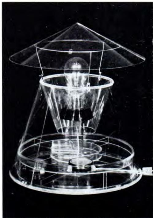
A transparent plastic light-trap designed to collect mainly soft-bodied insects, such as moths. The diameter at the base is 18 inches. The hood is only used during rain to protect the mercury vapour lamp. [Photo: C. Lourandos, C.S.I.R.O.]
