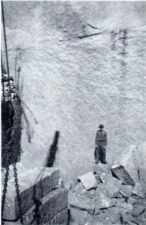
A working face in the granite quarry at Sodwalls, N.S.W. The large regular blocks are awaiting transport to Sydney, where they will be sawn into slabs. Note the small, closely-spaced drill holes (marked by white lines) along the upper edge of some of the blocks. A special type of chisel known as the "plug" is driven, between two short steel bars called "feathers", into each of these holes and the expansion of the "feathers" splits the block. [Photo: Author.]
