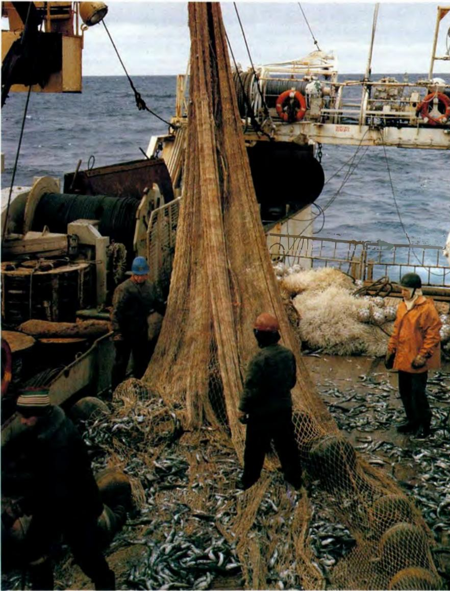
Remnants of a catch of icefish cover the deck of this Soviet trawler, fishing near Heard Island. The size of the net indicates the enormous capacity of these modern boats. Large bobbins are used to prevent the net from being snagged on the bottom.
