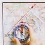
**2** Rotate the capsule until "N" on compass dial points north on map. North-South lines should be parallel with magnetic North grid lines on the map
