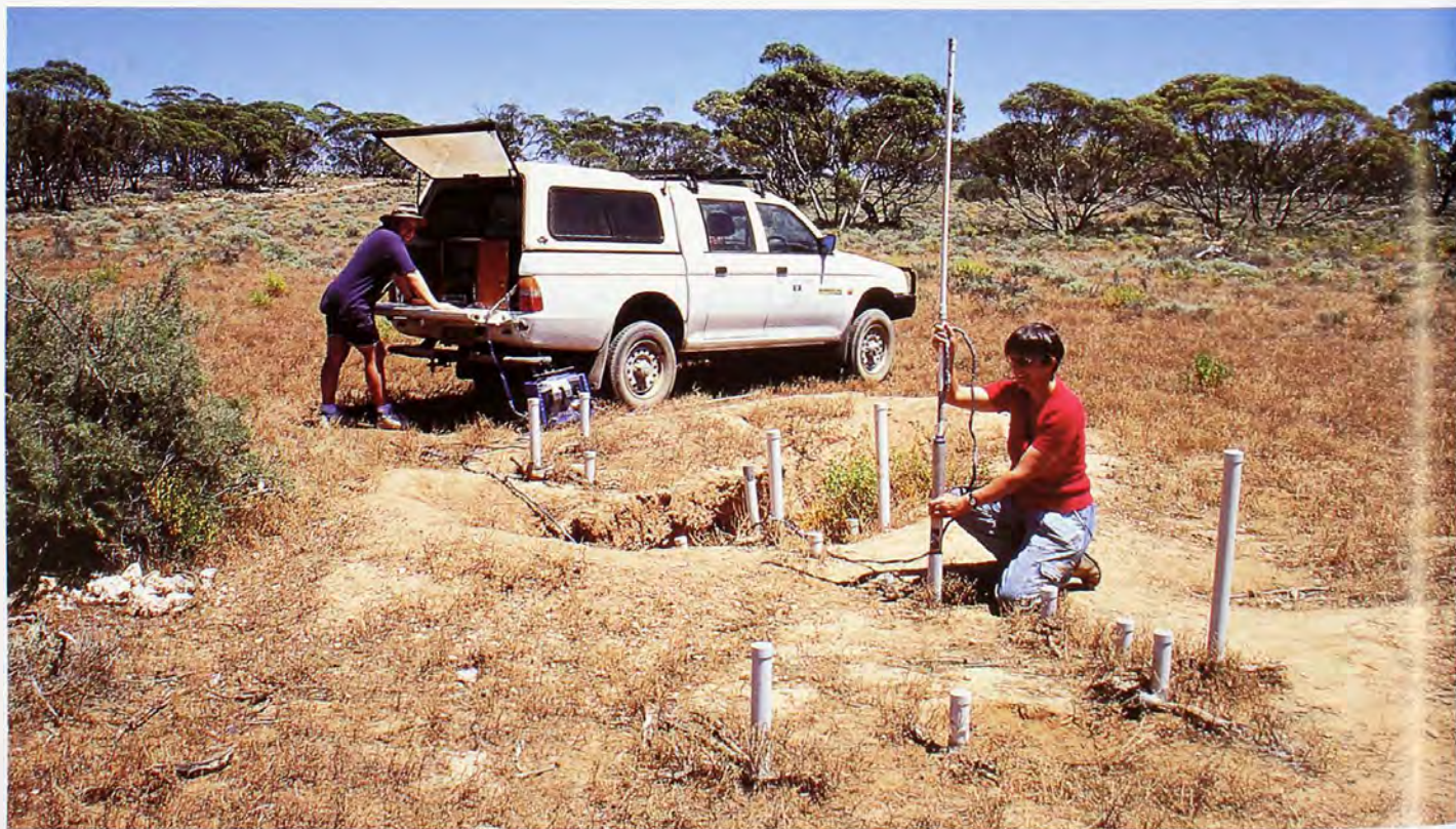
Wombat burrow interiors were viewed using a porthole camera lowered down PVC casings into the tunnel, with footage viewed and recorded on the surface.
