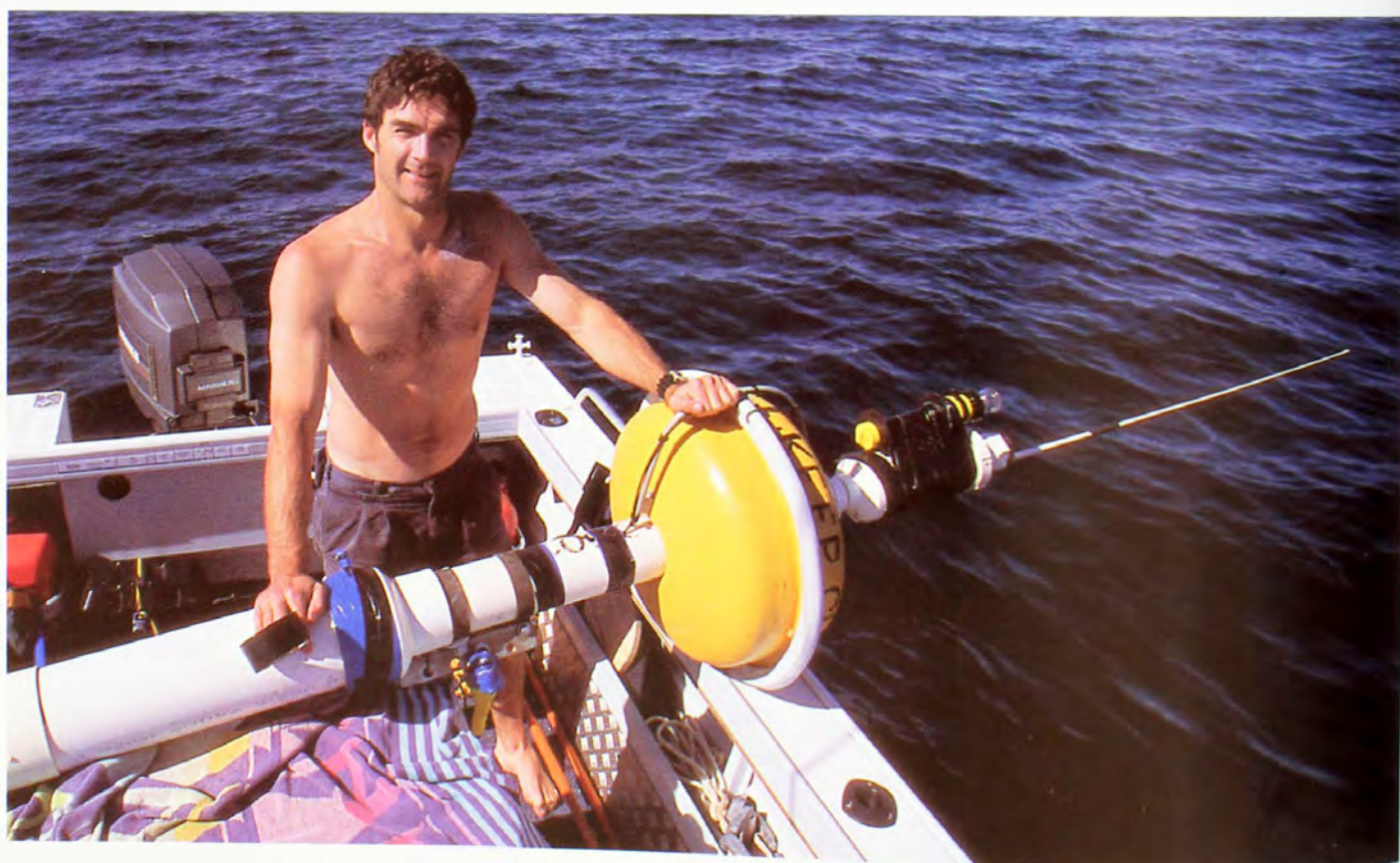
Whale songs are monitored using 'hydrophone-buoys'. These allow the sounds picked up by a hydrophone to be relayed back to a shore station in real time. This buoy is having its battery changed by the author off Peregrine Beach, Queensland.
