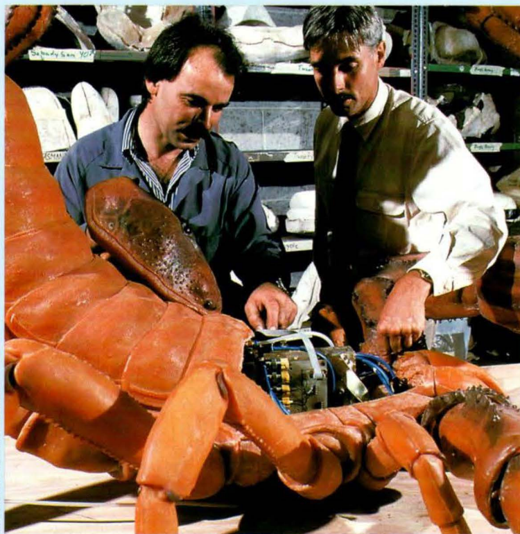
The scorpion at final stage of assembly having its animatronics tested. The next stage is the painting and finishing touches.
