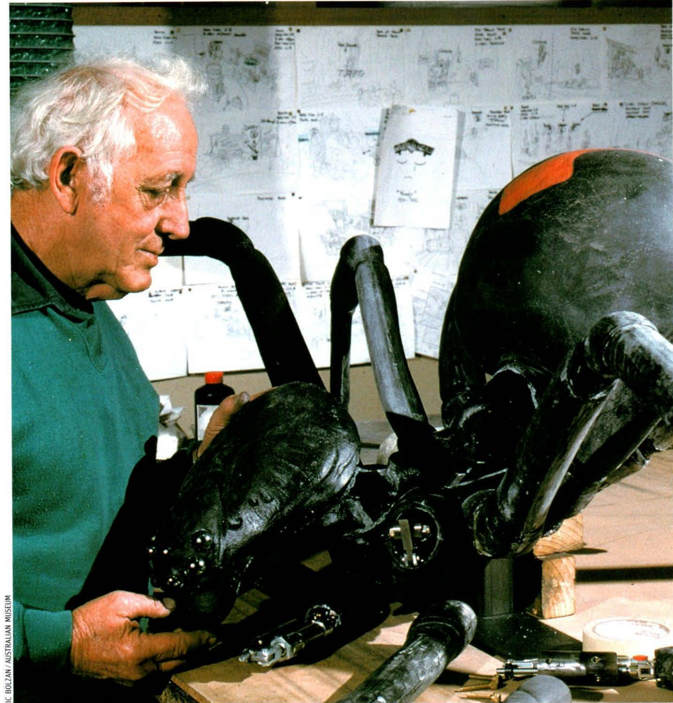
The Redback Spider model being assembled, with animatronics partially inserted.
