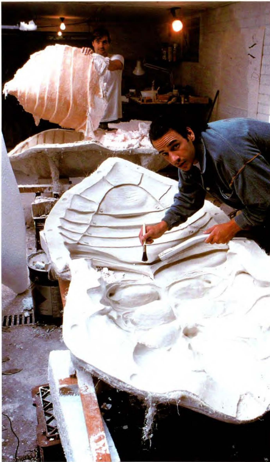
The polystyrene foam cicada body being released from its mould by Justin Robson (in background), while his assistant cleans out the other half. Justin's work may be familiar to many; it includes some amazing rice sculptures featured in a television commercial.
